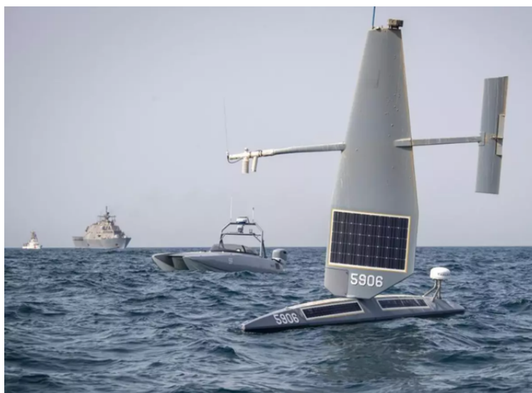
Figure 2. Explorer, a Saildrone (autonomous sailboat) that operates without a crew.
